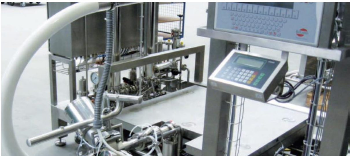
Container station with integrated scale and control system
